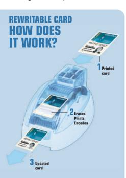
Tattoo RW is a ribbon-free printer that uses rewritable cards. Such cards contain a thermochromatic material that turns visible, or vanishes, according to the applied temperature. This reversible process makes it possible to erase and print on the same card up to 500 times. Your card turns into a powerful medium that displays temporary or updatable data such as bonus points and special offers on a loyalty card, or the name and relevant details of visitors on a corporate badge.
